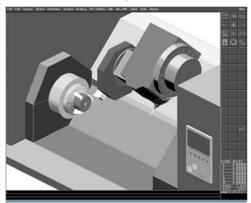
Camand Lathe has the ability to simulate the motion of the tool, holder, turret, and the part being cut.
