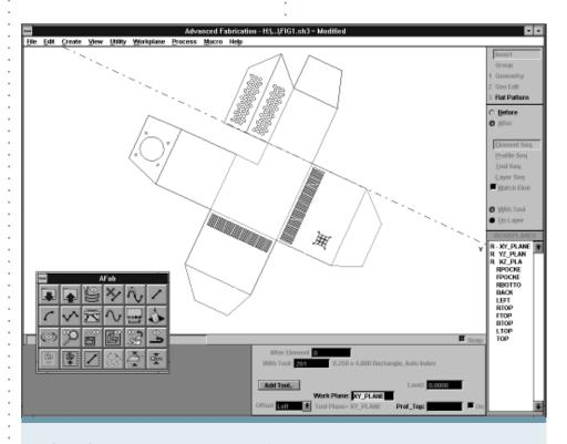
SmartCAM Advanced Fabrication unfolds a part in a single step.
