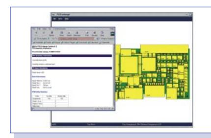
PCB.xchange allows you to preview IDF files and visualize the data exchange process. It provides rules-based filtering of components and features. In addition, you can generate Web-HTML reports of the PCB assembly.
