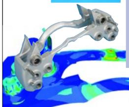
✓ Several new FE models were then created within I-DEAS<sup>®</sup> to evaluate their performance with the more detailed analysis parameters such as friction and mounting bolt interference. These models were used to drive the design of a completely new shape for the inboard beam. Instead of being totally curved, it now featured a straight portion in the critical areas, with three scallops to provide the necessary clearance for the adjoining bolts.
